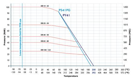
316L Body, Ends, Ball & Stem - Environment temperature [-50°C to +80°C] Ball with Upstream Vent Hole for Liquid Vaporization (One Way Valves)
