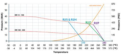
Carbon Steel Valve Minimum Temperature Limit: -10°C Environment Temperatures Range: [-55°C to +80°C]
