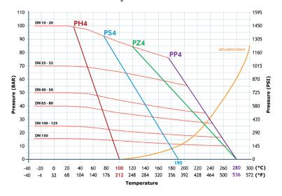
Carbon Steel Valve Minimum Temperature Limit: -10°C Environment Temperatures Range: [-55°C to +80°C]
